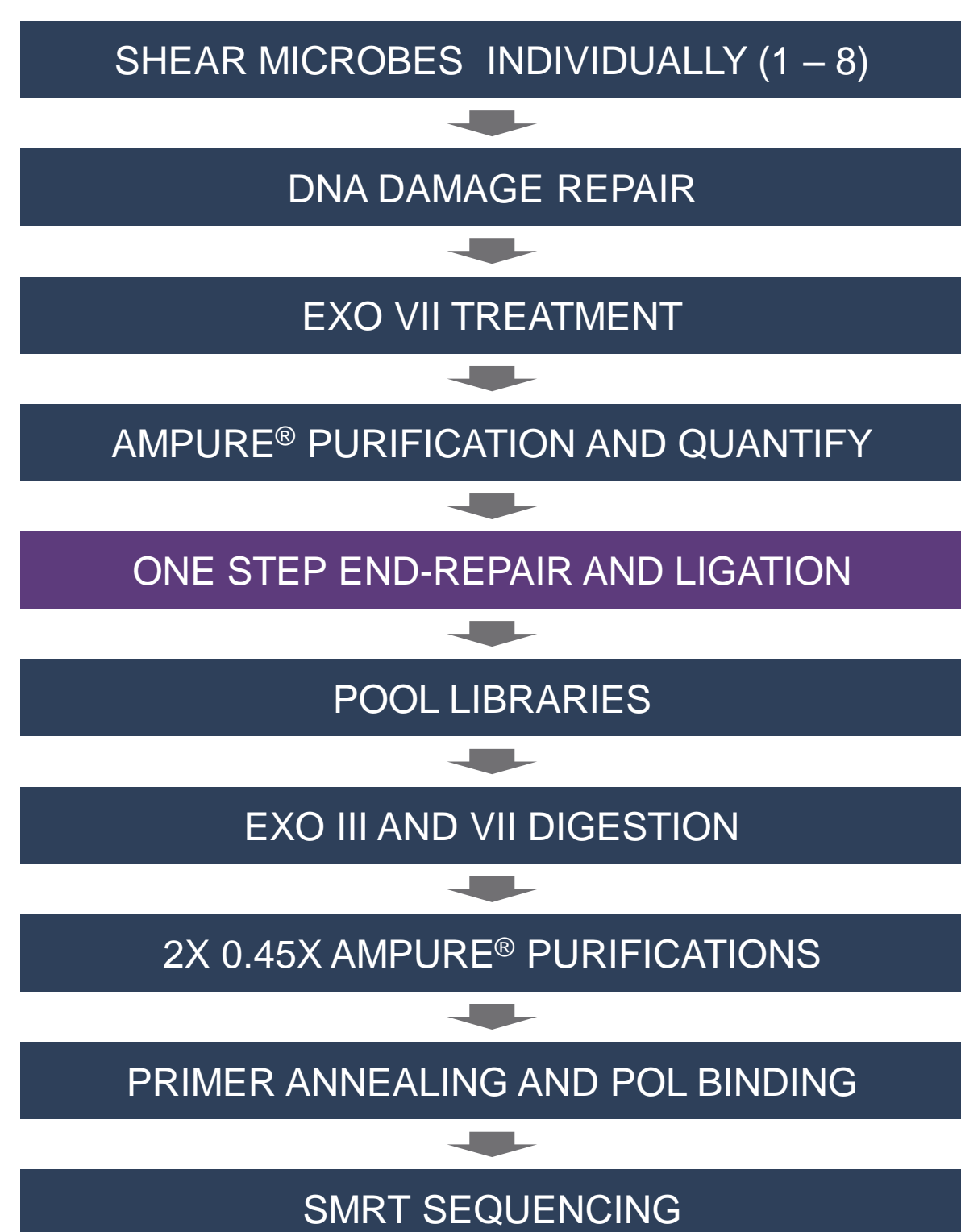
Fig. 1. Workflow for microbial multiplexing SMRTbell library preparation
