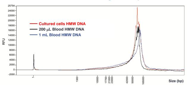
Example Femto Pulse DNA sizing QC analysis results for HMW DNA samples extracted with Nanobind HT kit using KingFisher Apex automation platform.
