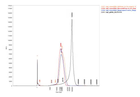
Figure 1. Agilent Femto Pulse electropherogram showing the size profile of HG002 genomic DNA unsheared (black), sheared on the Hamilton NGS STAR MOA system at 9  $ng/\mu$ L (orange), sheared on the Hamilton Microlab Prep system at 9  $ng/\mu$ L (red), and sheared on the Megaruptor 3 system at 35  $ng/\mu$ L (blue).
