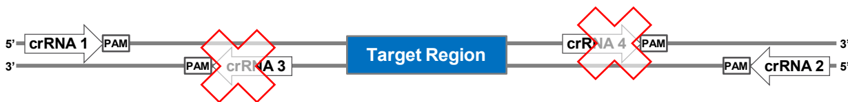
Figure 2. Illustration of four possible locations for crRNA designs for a generic target region. The two flanking crRNA designs for any target region must be located on opposite strands with the 3' end of each design closest to the target region. This will also place the PAM site in-between the crRNA design and the target region. Designs crRNA1 and crRNA2 are compatible with the No-Amp targeted sequencing procedure whereas designs crRNA 3 and crRNA 4 are not (shown crossed-out) as the 5' ends of these designs are closest to the target region with the PAM sites not adjacent to the target region.
