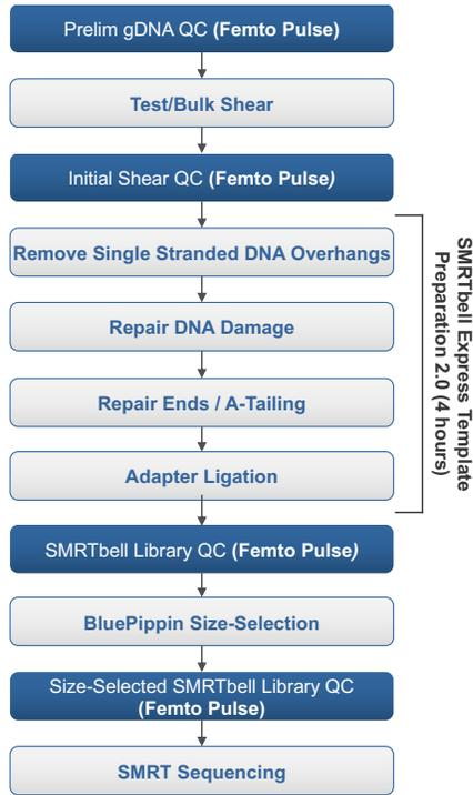
**Figure 1. Large-insert library construction workflow with SMRTbell Express Template Prep Kit 2.0.** Sizing with the Femto Pulse replaces all PFGE to complete critical QC checkpoints in less than 1.5 hours (blue boxes).
