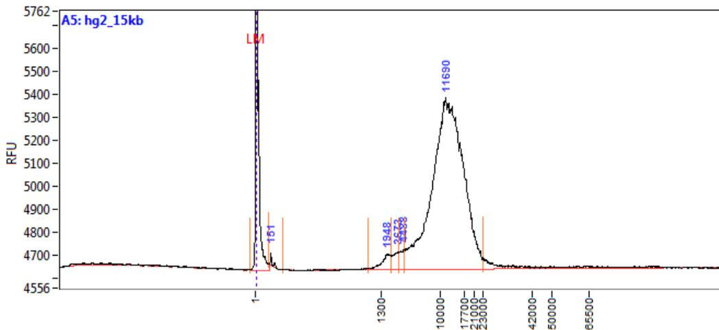
Figure 3: Example of human gDNA sheared to 12 kb using 15 kb shearing mode on the Megaruptor and evaluated on FEMTO Pulse.
