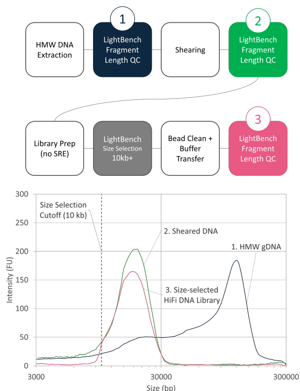
Figure 2 – Schematic of the integration of the LightBench® Discover in the CoLab's long-read sequencing workflow. Numbered positions indicate QC step performed by the LightBench® Discover (top). Electropherogram traces produced at each QC step (bottom). The vertical line indicates the location of the 10 kb size-selection cutoff.
