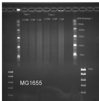
Dilutions of NGS-grade gDNA preps on pulsed-field gel. Most of the gDNA is over 20 Kb in length (mass middle is around 100 Kb).
