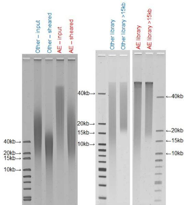
Pulsed-field gel electrophoresis demonstrated that gDNA from *E. coli* K12 strain MG1655 prepared by Amplicon Express (AE) was less fragmented than that from another commercial supplier (Other). Sheared AE gDNA also exhibited larger fragment sizes, as did SMRTbell libraries prepared from AE gDNA. No difference in library yield, either before or after size-selection, was seen (not shown).
