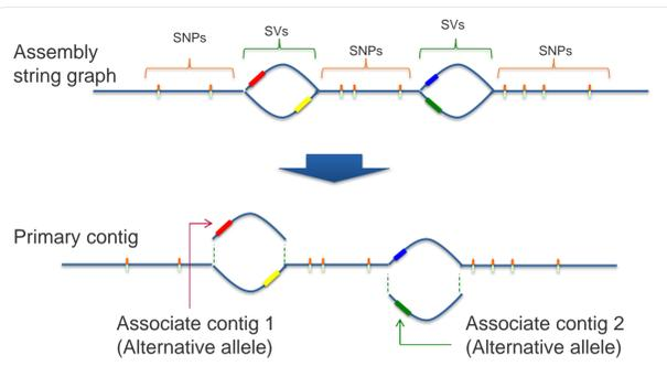
**Figure 4. Diploid Aware Contig Representation With Falcon.** During the assembly process, structural variants between haplotypes appear as 'bubbles' in the string graph. Falcon retains the long range information, while maintaining the relationship between the alternative alleles in the form of associate contigs.
